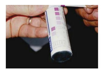
Example of a nitrate quick-test: this particular test showed that drinking water well had a very high level of nitrate
