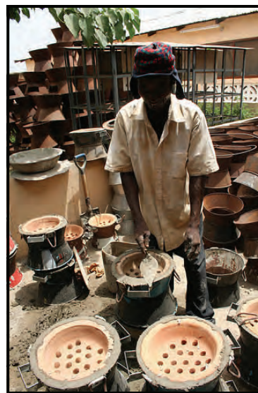
Toyola employee assembling stove bodies and liners
