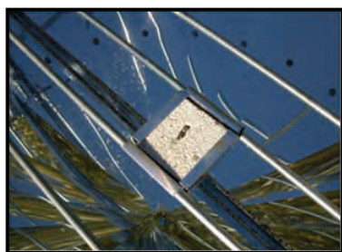
Detailed view of pot bottom sensor. Note the reflective casing protecting the cellular concrete.
