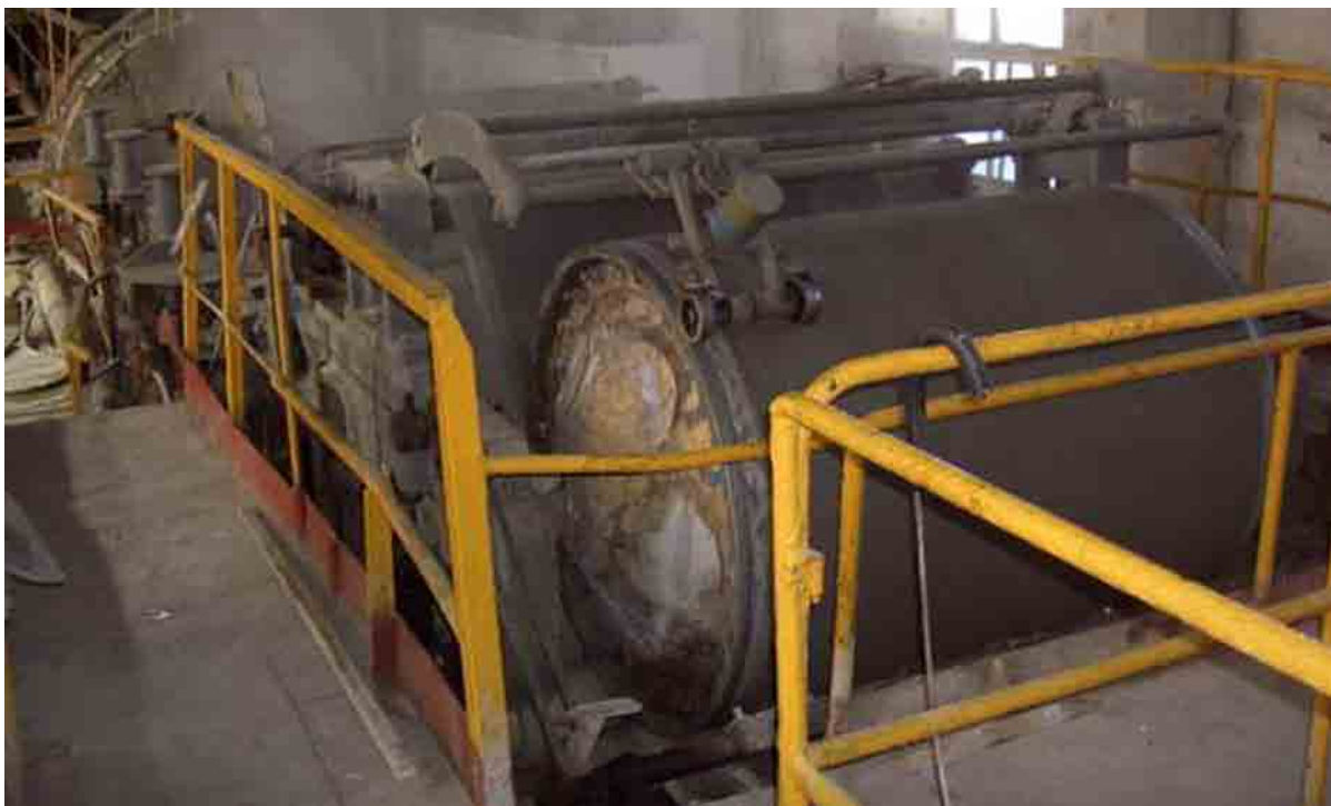
Forming of roofing slates
