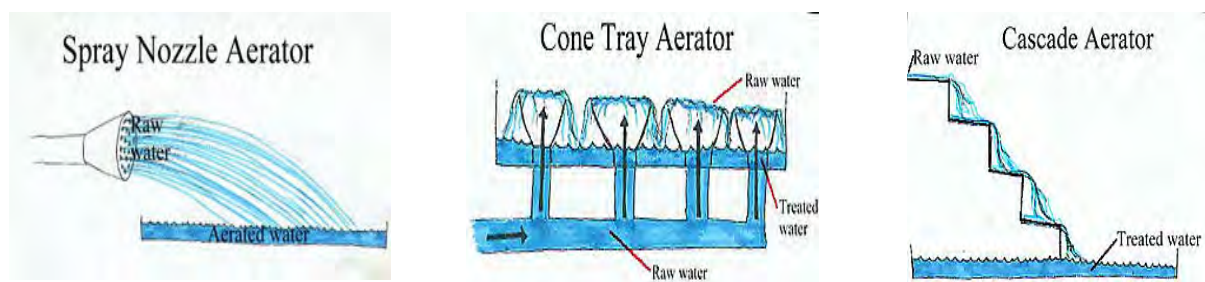
Figure 2: Drawings of different technical devices used for aeration
