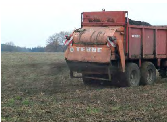
Application of dewatered sewage sludge on agricultural field in Germany
