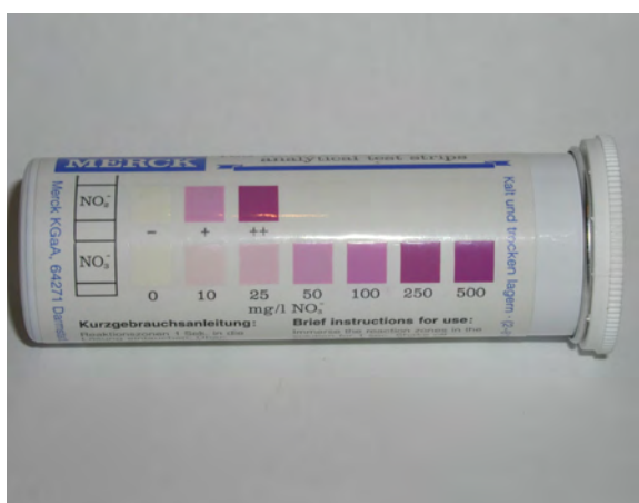
Nitrate pollution can quickly be detected in water samples by using nitrate test strips
