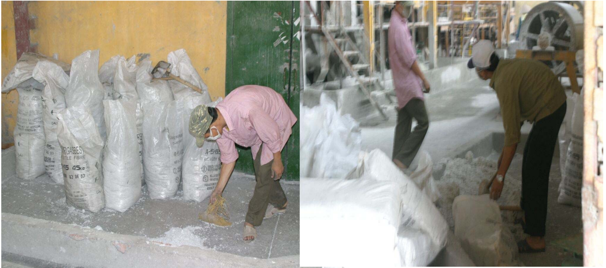
Worker Sweeps Asbestos Fibers
