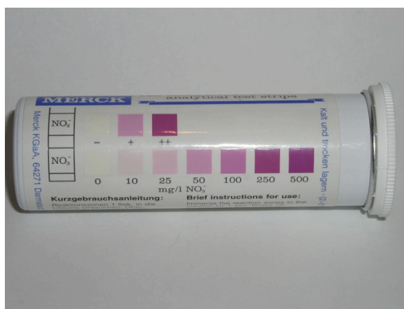
Nitrate testing tube containing test strips, measuring the nitrate concentration of water with a range from 0 – 10 – 25 – 50 – 100 – 250 – 500 mg/litre are very suitable.
