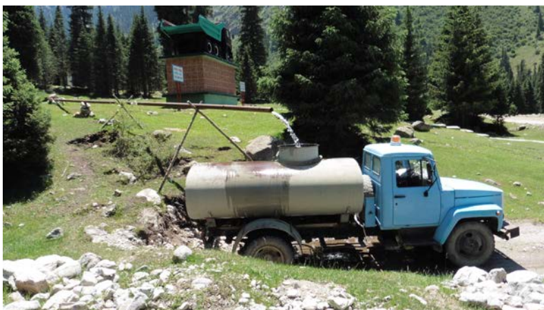
A common method for delivering water to a community immediately after an emergency has happened, is water tankering
