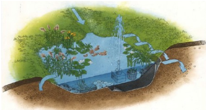
Simple pond scheme for rainwater retention
